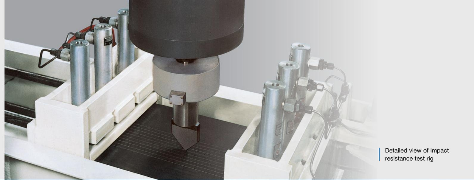
Detailed view of impact resistance test rig
