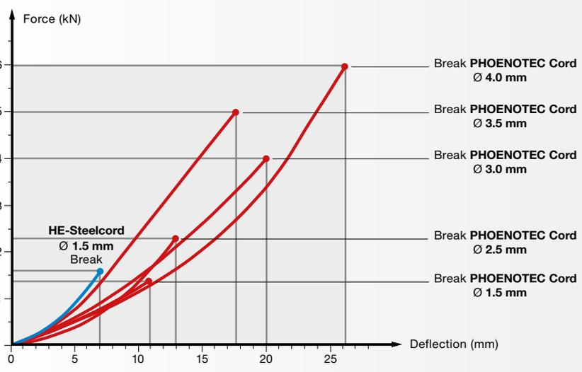
Force/elongation behaviour of different PHOENOTEC cords and of a high elongation (HE) steel cord, embedded in rubber and loaded at right angles to their longitudinal axis
