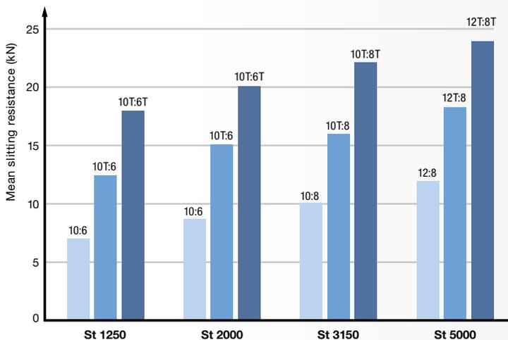
**Effect of double PHOENOTEC with different types of PHOENOCORD conveyor belts.**
