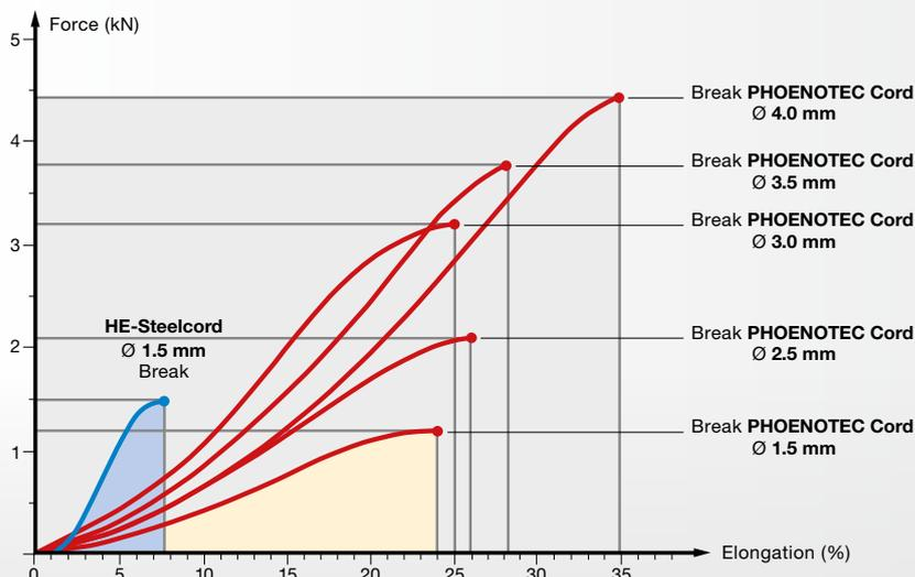
**Force/elongation behaviour of different PHOENOTEC cords and of a high steel cord, loaded in axial direction**
