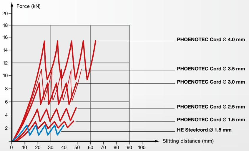
Force/elongation PHOENOTEC cords and of HE steel cord assemblies, embedded at right angles to their longitudinal axis
