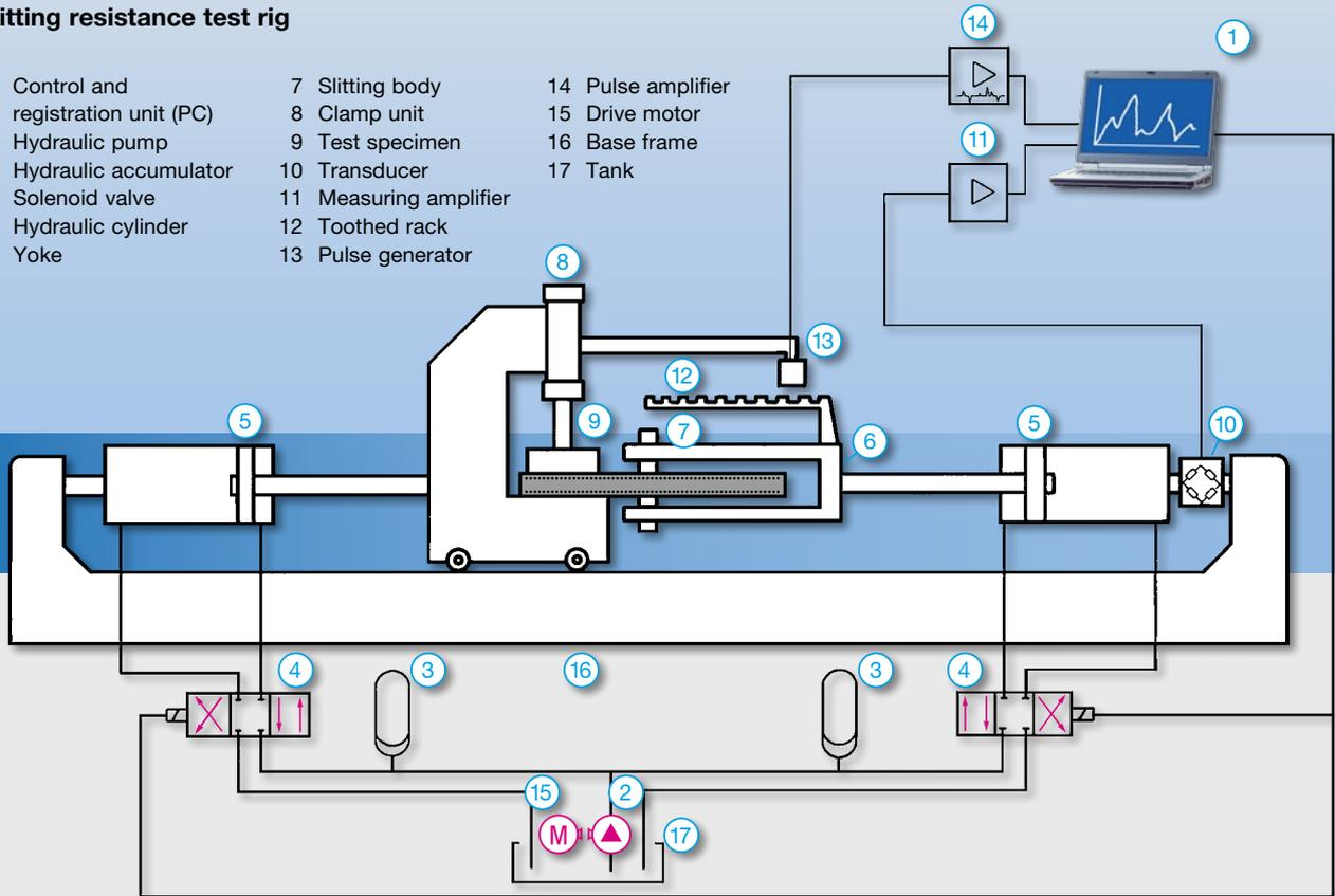
During the slitting operation, with the aid of an electrodynamic pulse generator (13), the toothed rack (12) produces a pulse sequence which depends on the tooth pitch and the slitting speed and which is recorded with the aid of pulse amplifier (14) and registration unit. The slitting speed can be easily calculated by the PC and registered for each individual test.
