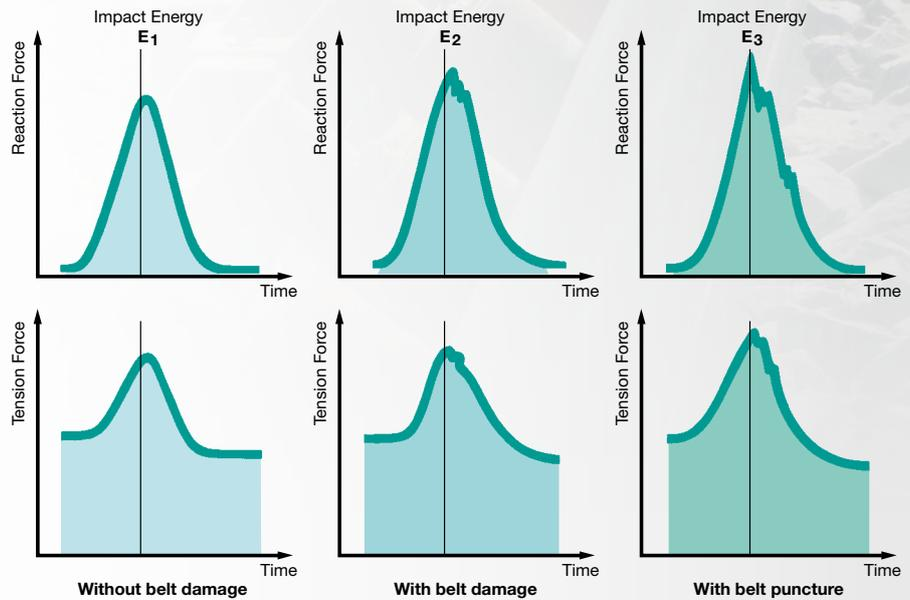
Impact resistance in dependence on pretension (% of minimum belt breaking strength)
