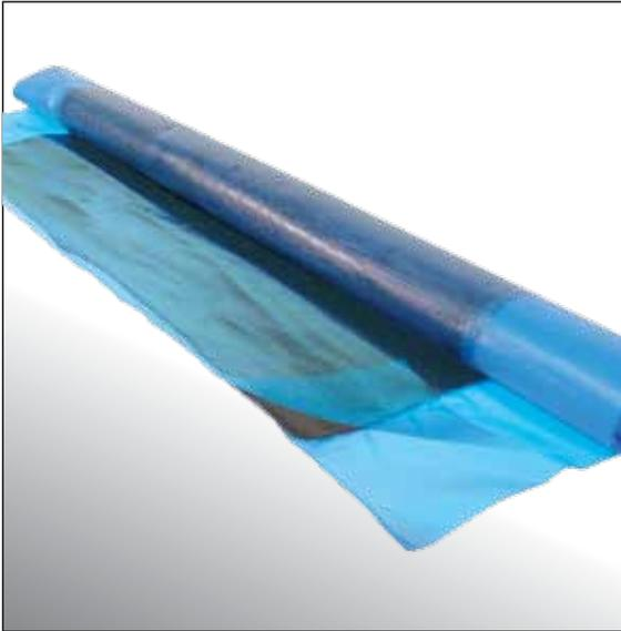
Skimmed Breaker Fabric is a Leno Weave RFL treated fabric skimmed with uncured rubber for hot vulcanized belt splicing reinforcement. It is designed for use in step splicing and finger splicing of standard grade fabric belts
