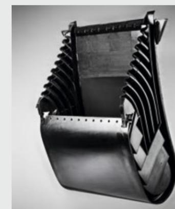
The belt consists of two PHOENOCORD belt stripes which are connected by strong rubber covered cross traverses. The material is carried by fabric reinforced rubber buckets, which are mounted to the cross traverses. All three components are connected threaded joints which allow quick and easy installation.
