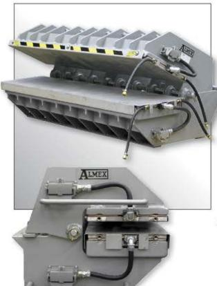
The Almex Edge Repair Press is designed to restore belt edges to their original quality. Increasing the integrity and life of the conveyor belt and the systems it comes in contact with.
