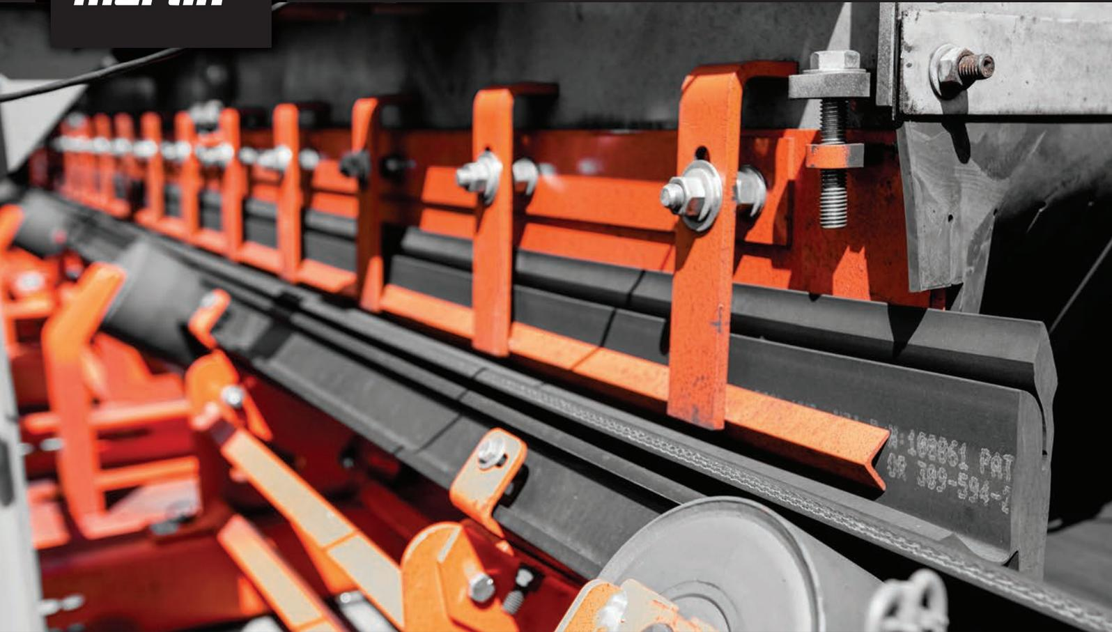
*A crucial requirement in any transfer point designed for reduced spillage and high efficiency is an effective sealing system at the edge of the belt. An effective sealing system incorporates multiple components to not only prevent spillage, but also protect the system from material-load forces.*
