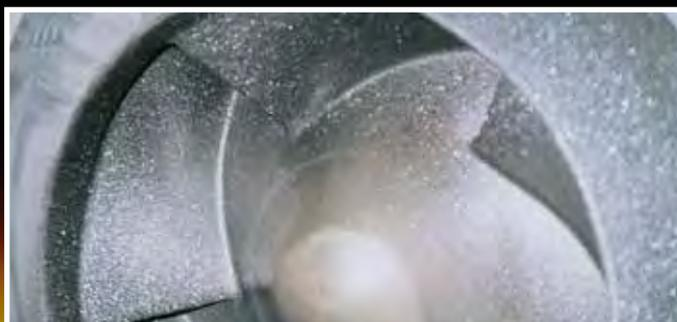
Impeller made of SICcast®
