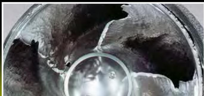
Impeller made of Duplex Stainless Steel
