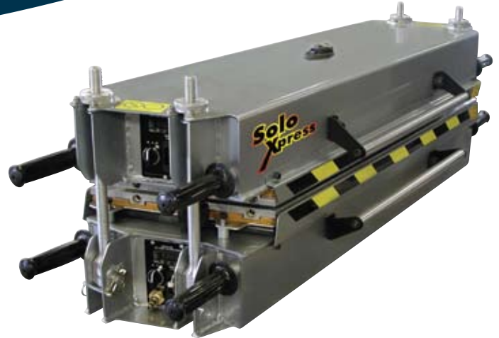
Solo Xpress Model 100-1337T1F with inset T1F control panels
