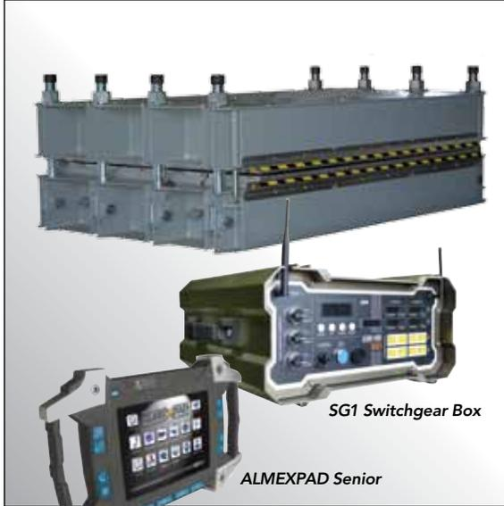
Customized and rugged, these two-piece frame presses offer simplified assembly, reducing set-up time. Frame presses are well-suited for large, open sites. Use RAB and AB for on-site splice stations or where overhead cranes are available. Built with unmatched Almex technology, RAB and AB frame presses are constructed with the following proven components:
