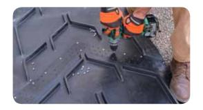
The ISC® splice allows the belt to be installed by simply screwing both ends together without overlap or extra thickness. This system guarantees an immediate installation with less down time.
