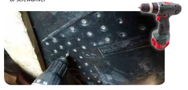
A REAL INNOVATION IN THE CONVEYOR BELT LACING INDUSTRY. WE VULCANIZE ISC® SPLICE INTO THE BELT OF YOUR CHOICE IN OUR WORKSHOP, YOU JUST NEED TO POSITION THE BELT AND SCREW BOTH ENDS TOGETHER!
